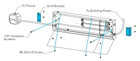
Note: this product can be installed in recessed ceilings if proper access and spacing criteria is met. In recessed or non-recessed installations, keep insulation, building members, and other driver enclosures at least 3 inches (76mm) away from all sides of the enclosure.
