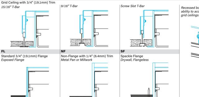
Recessed box allows for 1/2" of adjustability to accommodate a variety of grid ceilings
