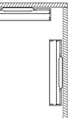
The canopy can be installed either below the ceiling plane or semi-recessed into the ceiling for a flush mount installation
