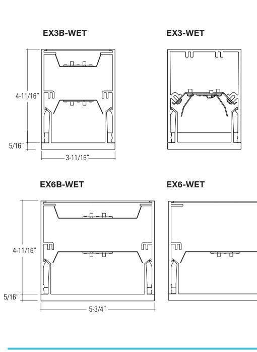
EDGE Wet is available in a 3" and 6" aperture in both direct and bidirectional light distributions. Choose from recessed, wall, surface or pendant mounting options and 4 standard color finishes. Housing is the same for recessed and suspended.
