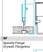
Recessed box allows for 1/2" of adjustability to accommodate a variety of grid ceilings
