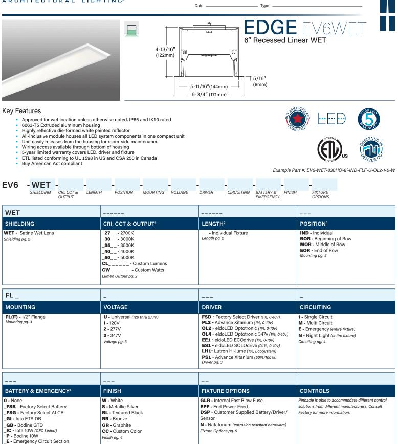
"When specifying OUTPUT the first \_ is for specifying either 8 - 80CRI or 9 -90CRI. The ending \_ are for specifying output, example HO - High Output. See output charts for more information. <sup>2</sup>Individual fixtures come in nominal 2, 3, 4, 5, 6, 7, & 8' lengths, see pg. 2 for actual lengths. <sup>3</sup>Specify position of fixture. Use IND for an individual fixture, use BOR, MOR, or EOR for building connected rows. <sup>4</sup>Enter quantity for Battery and Emergency, Example 2P.
