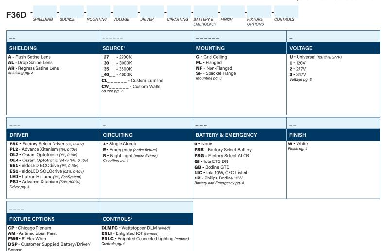
1When specifying SOURCE the first \_ is for specifying either 8 - 80CRI, 9 - 90CRI. The ending \_ \_ are for specifying output, example HO - High Output. See output charts for more information. 2Controls can only be used with Single Circuit (1) or Emergency Circuit (E), cannot be used with any battery options. See Controls chart on page 4 for driver options and more information.
