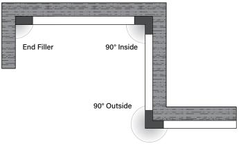
All fixture lengths within a pattern will be rounded to the nearest foot. End fillers and Corners (both field cut) will be used to complete the pattern. Factory Drawings will reflect all fixture, corner, and end filler locations and will need to be approved before an order is entered.
