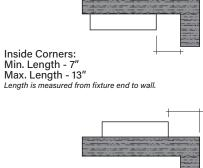
Outside Corners: Min. Length - 0" Max. Length - 9-1/2" Length is measured from fixture end to wall.
