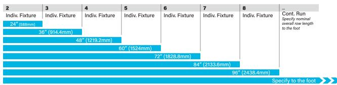
Fixture lengths do not include endcap dimensions. See bullet points listed above for each endcap. Example: 2' fixture (24") + 2 Standard Flat Endcaps (5/8") = 24 5/8" overall.
