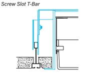
Recessed box allows for 1/2" of adjustability to accommodate a variety of grid ceilings
