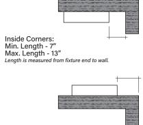
Outside Corners: Min. Length - 0" Max. Length - 9-1/2" Length is measured from fixture end to wall.
