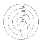
For all available IES files, please visit our website at pinnacle-ltg.com. Photometry testing in accordance to IESNA-LM-79-08 at an NVLAP accredited testing laboratory. Testing conducted at 25°C ambient conditions
