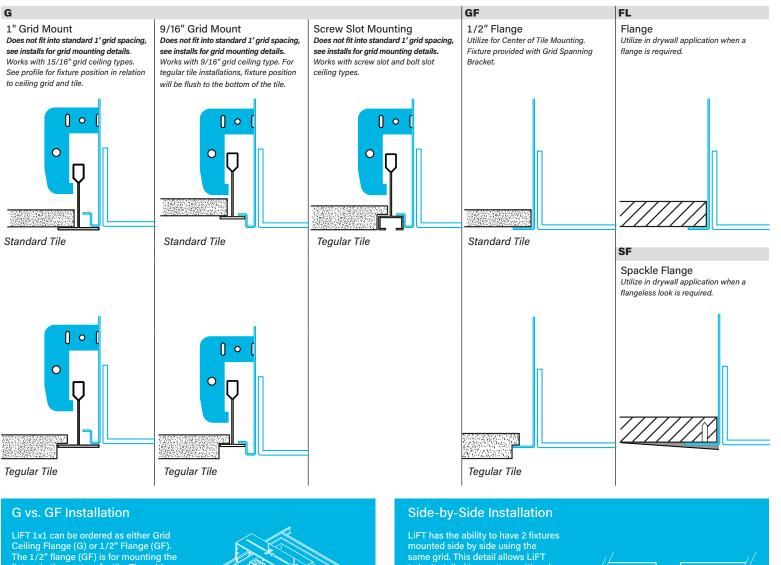
Ceiling Flange (G) or 1/2" Flange (GF). The 1/2" flange (GF) is for mounting the fixture in the center of a tile. The grid ceiling flange (G) is for if you are making a pattern with LiFT and would want to mount this off center. The GF mounting option comes with a grid spanning hold the fixture in the center of the tile.
