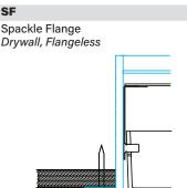
Recessed box allows for 1/2" of adjustability to accommodate a variety of grid ceilings
