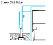
Recessed box allows for 1/2" of adjustability to accommodate a variety of grid ceilings
