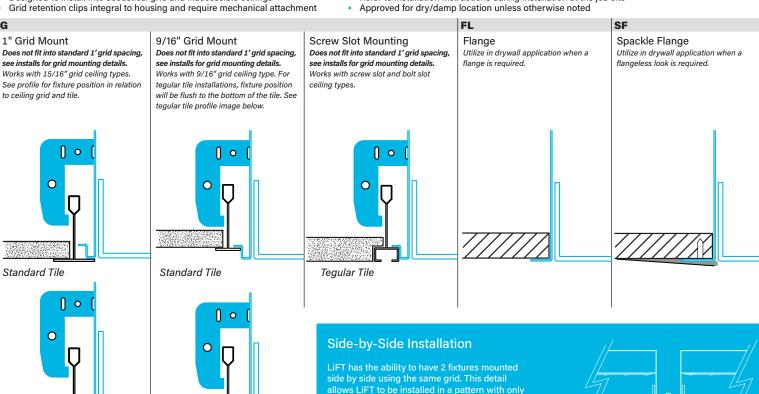
the space of the T-bar between the fixtures.
