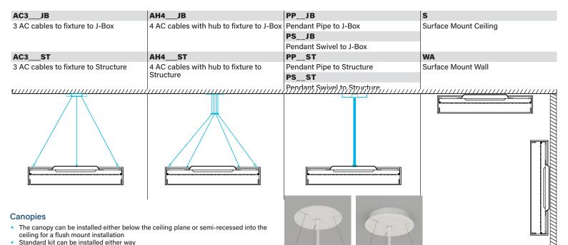
Flush canopy installation is not available for fixtures installed below a grid rail
