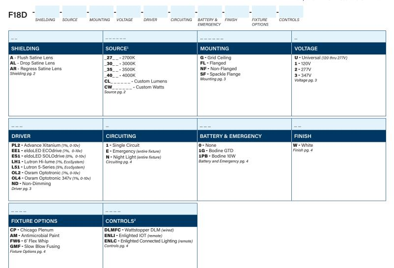
When specifying SOURCE the first \_ is for specifying either 8 - 80CRI, 9 - 90CRI. The ending \_\_ are for specifying output, example HO - High Output. See output charts for more information. <sup>2</sup>Controls can only be used with Single Circuit (1) or Emergency Circuit (E), cannot be used with any battery options. See Controls chart on page 4 for driver options and more information.
