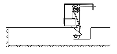
1. Insert thin tool between housing and lens.
