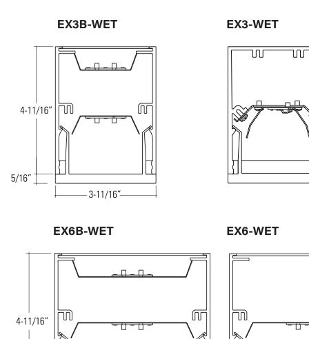
EDGE Wet is available in a 3" and 6" aperture in both direct and bidirectional light distributions.
