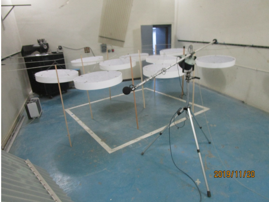
Figure 1 – Specimen mounted in test chamber
