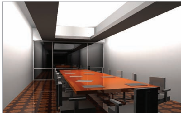
Combination Indirect Cove and Wall Wash
